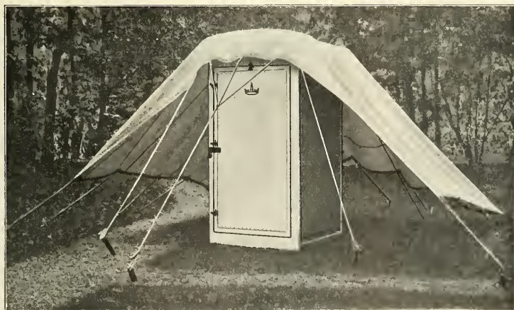
Small Torsion Balance with sun tent. (Courtesy of The American Askania Corporation, Houston, Texas.)
